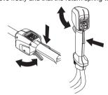
See instructions under the Start heading. Start the machine and apply full power. Release the power trigger and check that the cutting attachment stops and remain at a standstill.
