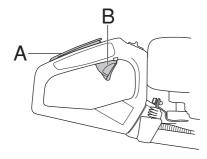
Make sure the throttle control is locked at the idle setting when the throttle lock is released.
