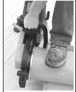
Align proper SpeedMill Bowl with end of pipe, and move toward the pipe so that the pipe is slightly beveled. Note: The bevel required is usually quite small, so do not remove excessive pipe material.
