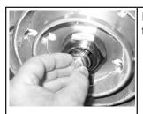
Install the blade shaft bolt into the Hub Assembly.
