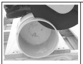
Move saw forward while maintaining a "square cut" on the end of the pipe. This means the cut should always be perpendicular to the length of the pipe.
