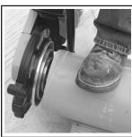
Bevel Pipe: Position SpeedMill Bowl near end of pipe to be beveled. Accelerate power cutter to full throttle.
