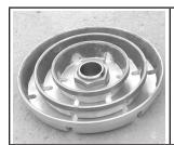
Unwrap SpeedMill bowl / Hub Assembly from the packaging. Initially all three sizes of SpeedMill Bowls (4", 6", 8") are assembled to the Hub Assembly.
