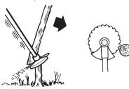
To fell a tree forwards, the bottom of the tree should be pulled backwards. Pull the blade backwards with a quick, firm movement.
