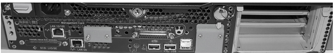
Figure 3-3 HP 9000 rp3410/rp3440 Server - Rear View
