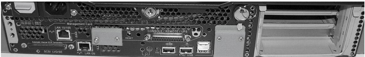
Figure 1-3 HP 9000 rp3410 and rp3440 Servers - Rear View
