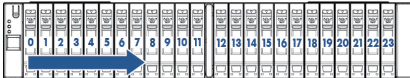
Figure 86 HP M6710 Drive Enclosure (2U24) Disk Drive Placement Order
