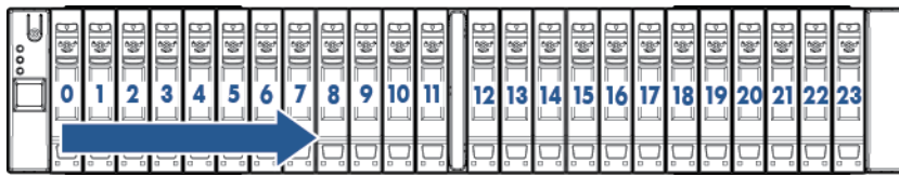
Figure 22 HP M6710 Drive Enclosure (2U24) Disk Drive Placement Order
