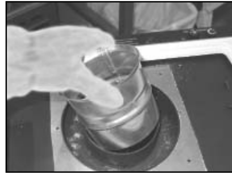
Figure 8.3 Remove the inner collar adapter.
