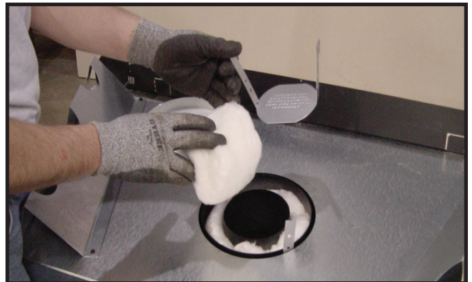
Figure 7.5 Remove the insulation basket and white insulation from the center vent pipe.
