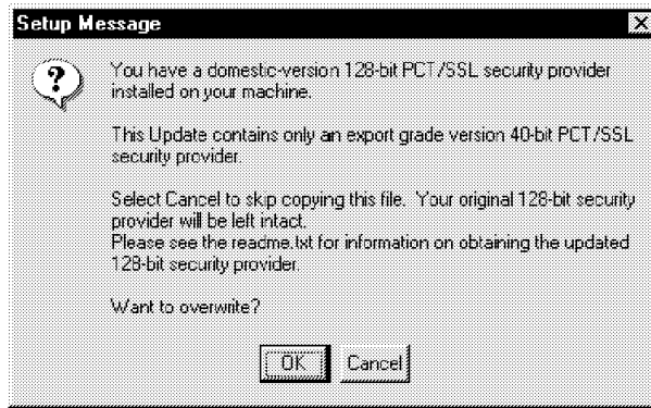
Figure 124. Encryption Components in the Service Pack. If you use 128-bit encryption, you should click on Cancel in order not to overwrite the encryption files.
