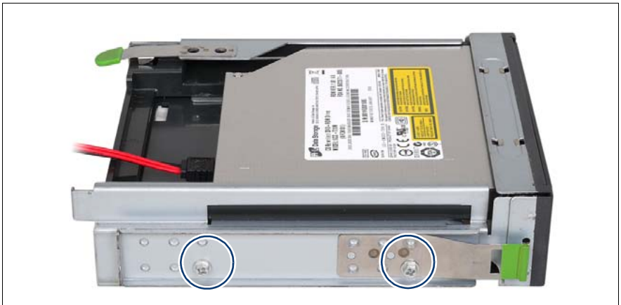
Figure 36: Attaching EasyClick rails to Multibay 1
