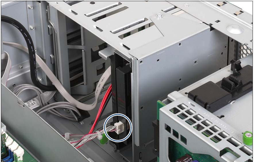
Figure 41: Connecting the I 2 C cable to the LSP/LSD
