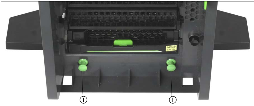
Figure 82: Locking buttons engaging
