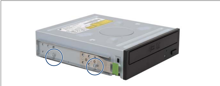
Figure 28: Attaching the EasyClick rails - example: DVD drive
