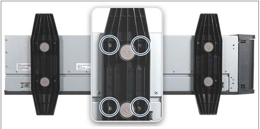
Figure 6: Removing the server feet
