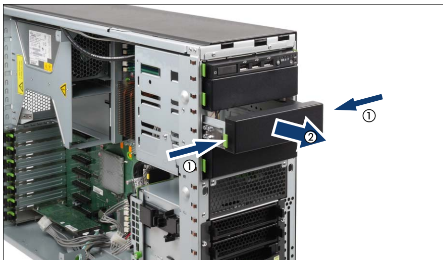
Figure 26: Removing the dummy cover
