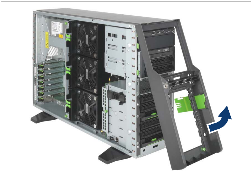
Figure 5: Removing the front cover
