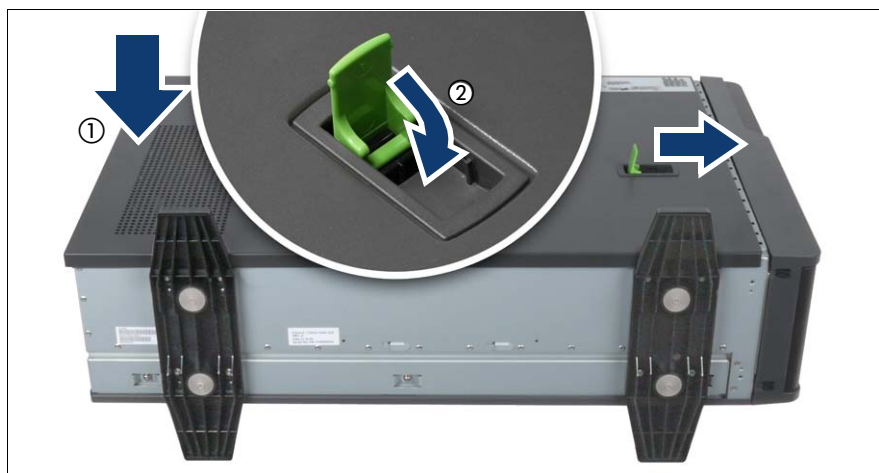
Figure 84: Closing the server
