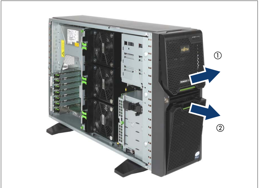
Figure 3: Removing the drive cover and the HDD cover
