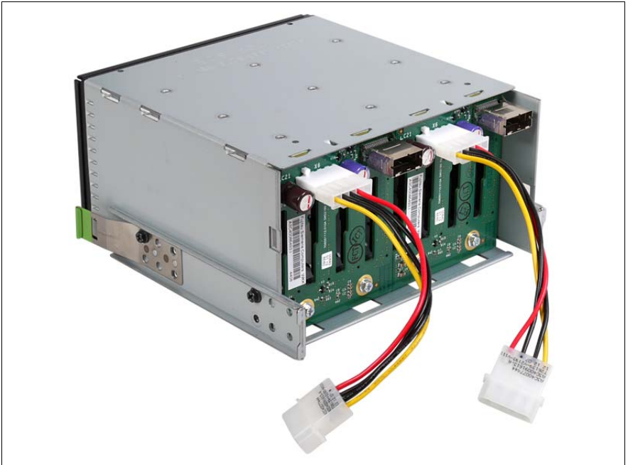
Figure 46: Connecting PS adapter cable to HDD backplanes
