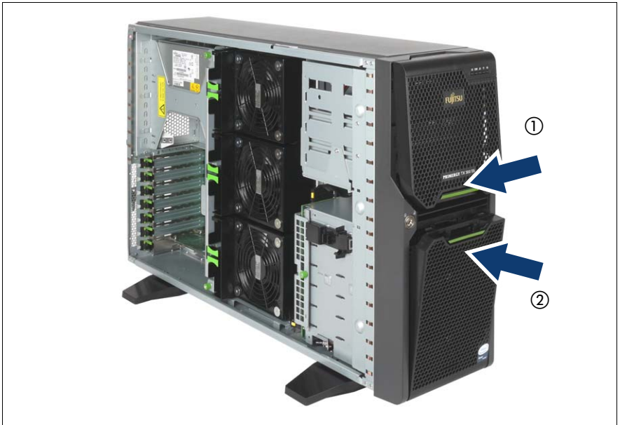
Figure 83: Attaching the HDD cover
