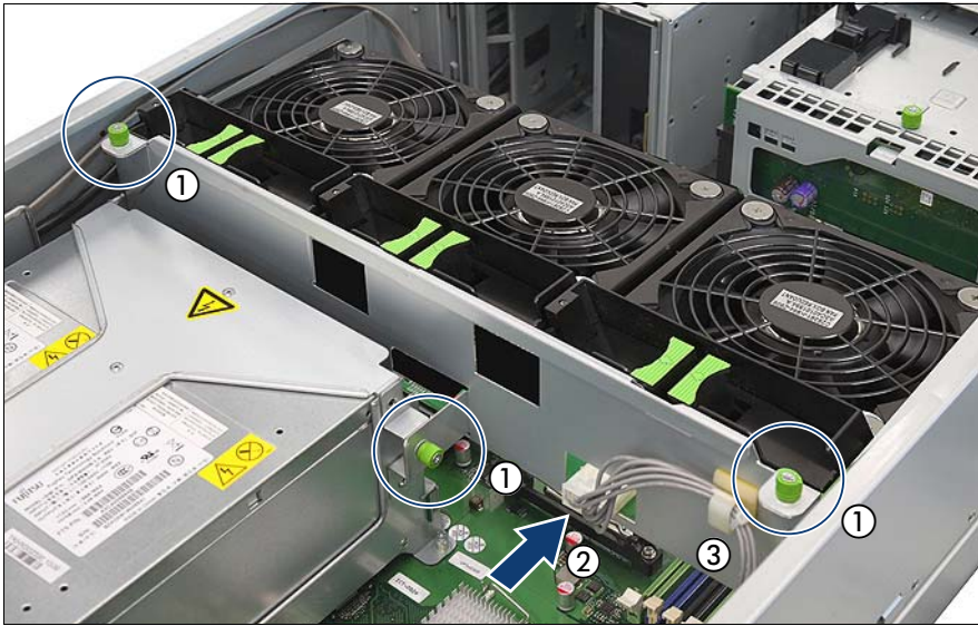
Figure 79: Connecting the power cable
