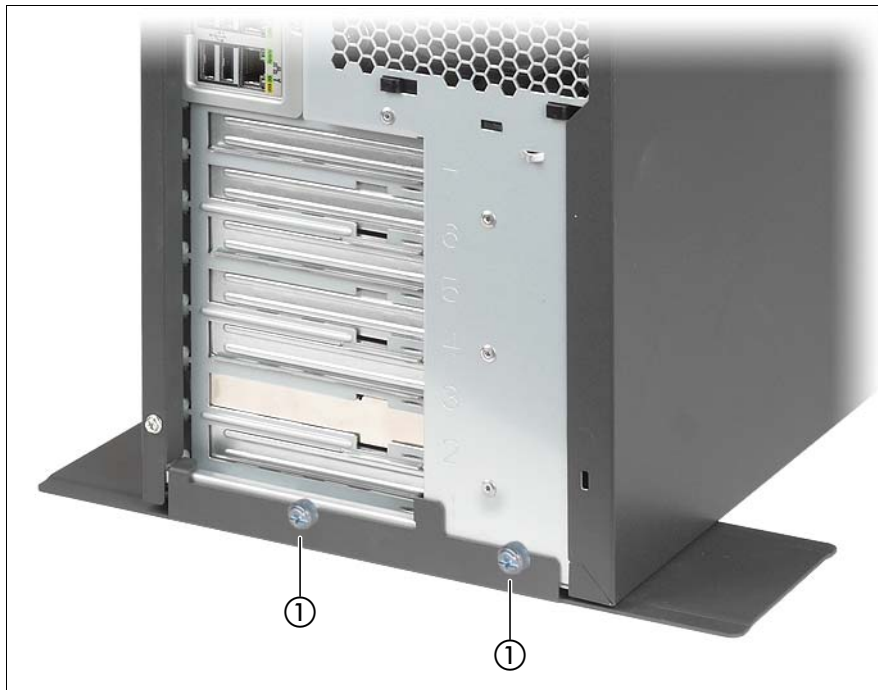
Figure 2: Mounting the anti-tilt bracket
