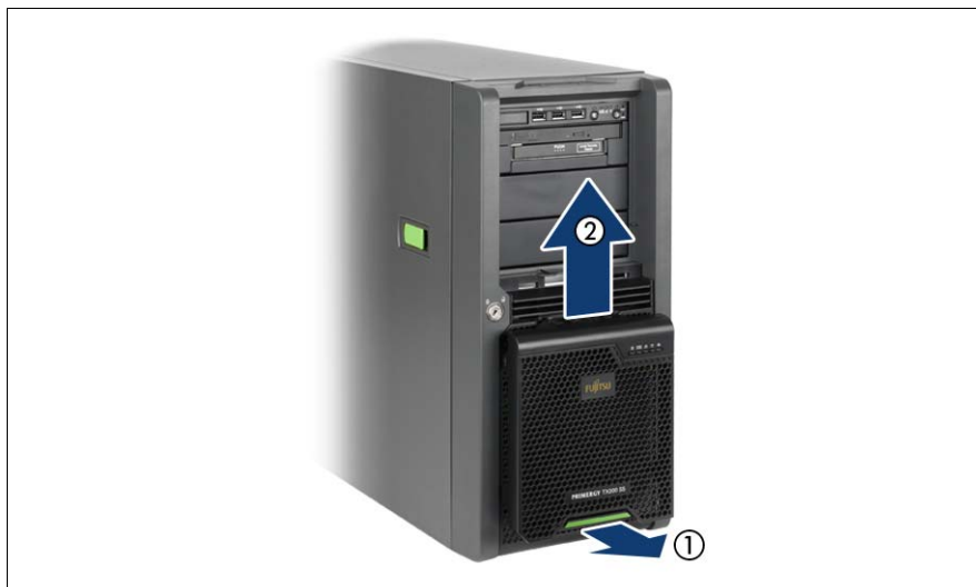
Figure 13: Removing the drive cover from the hard disk drive cover
