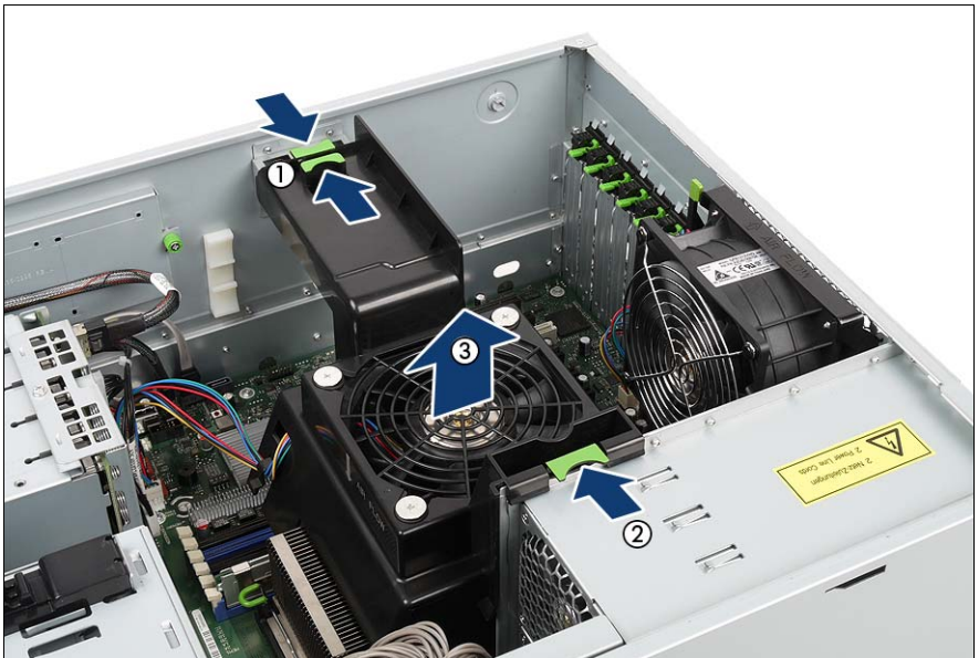
Figure 29: Example: Removing system fan 2&4
