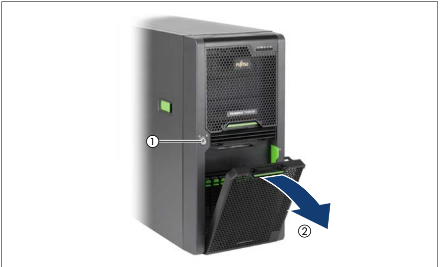
Figure 14: Removing the hard disk cover
