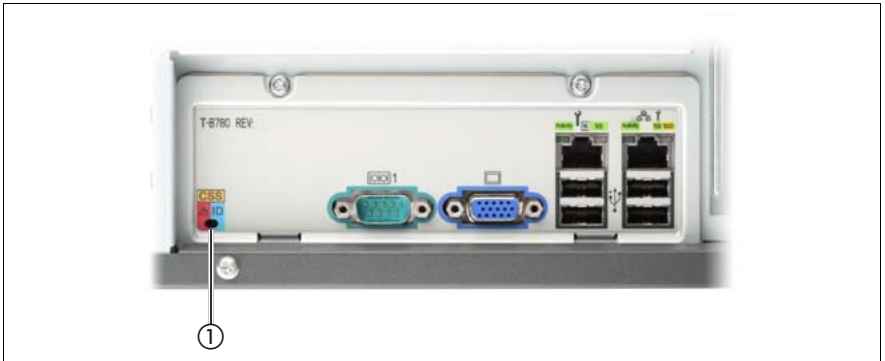
Figure 17: Indicators on the connector panel: CSS, Global Error and ID indicators
