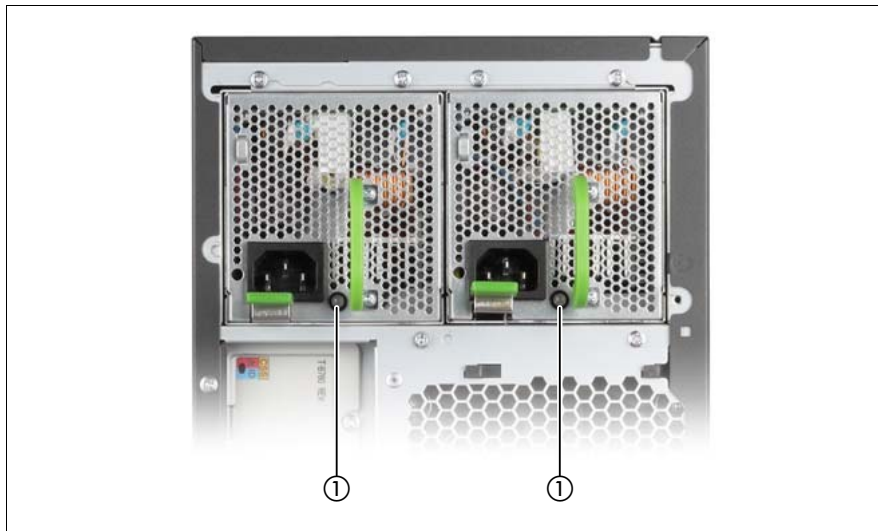
Figure 19: Indicators on the hot-plug power supply units
