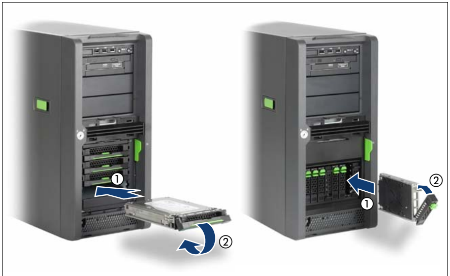
Figure 26: Installing the 3.5-inch and 2.5-inch HDD modules
