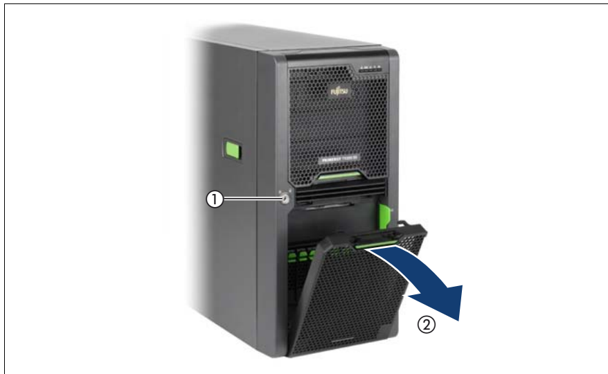
Figure 23: Removing the hard disk cover
