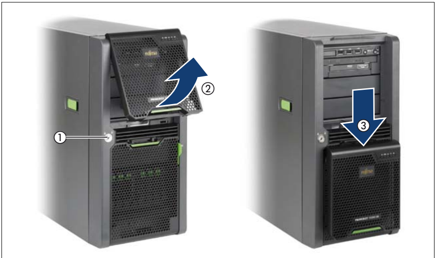
Figure 12: Removing the drive cover and snapping it into the hard disk drive cover
