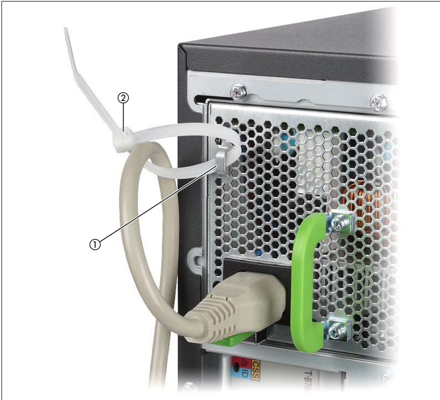
Figure 11: Using cable ties
