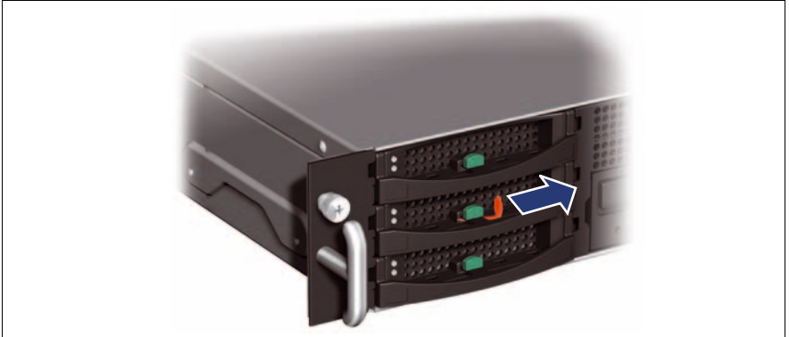
Figure 19: Removing the transport lock
