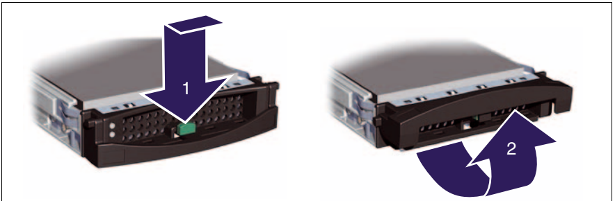
Figure 20: Unlocking the HDD module
