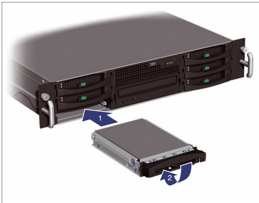
Figure 21: Installing the HDD module
