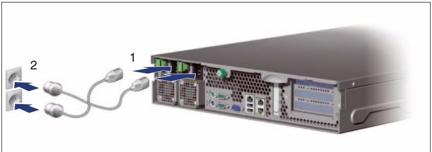
Figure 10: Connecting the server to the mains
