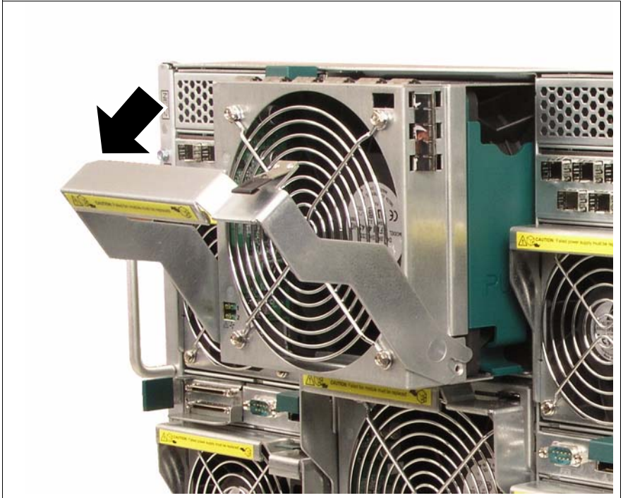
Figure 84: Removing the fan unit
