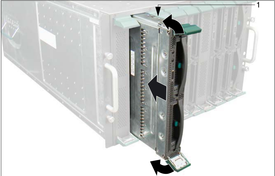
Figure 32: Inserting the server blade
