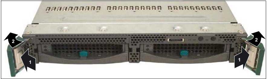
Figure 31: Turning the eject handles into the unlocked position (2-way server blade)
