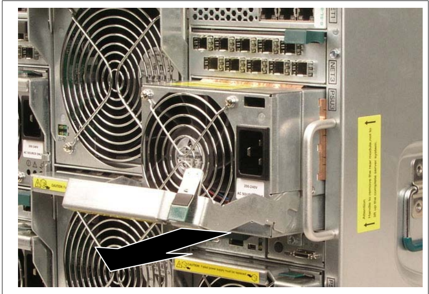
Figure 79: Removing the PSU
