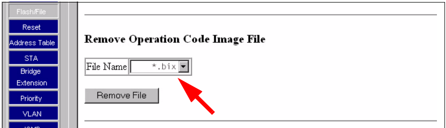
Figure 24: Removing an operation code image file
