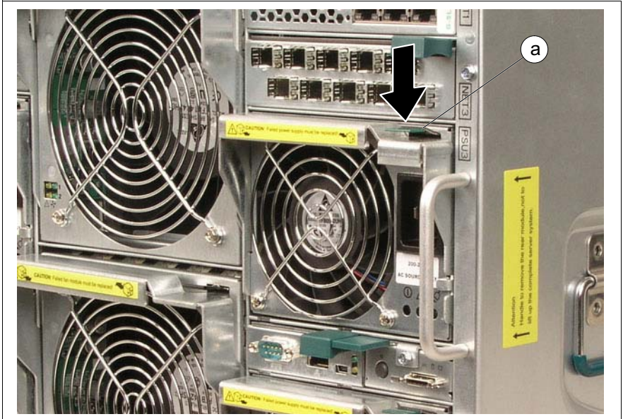
Figure 77: Disengaging the power supply unit (a = green touch point)
