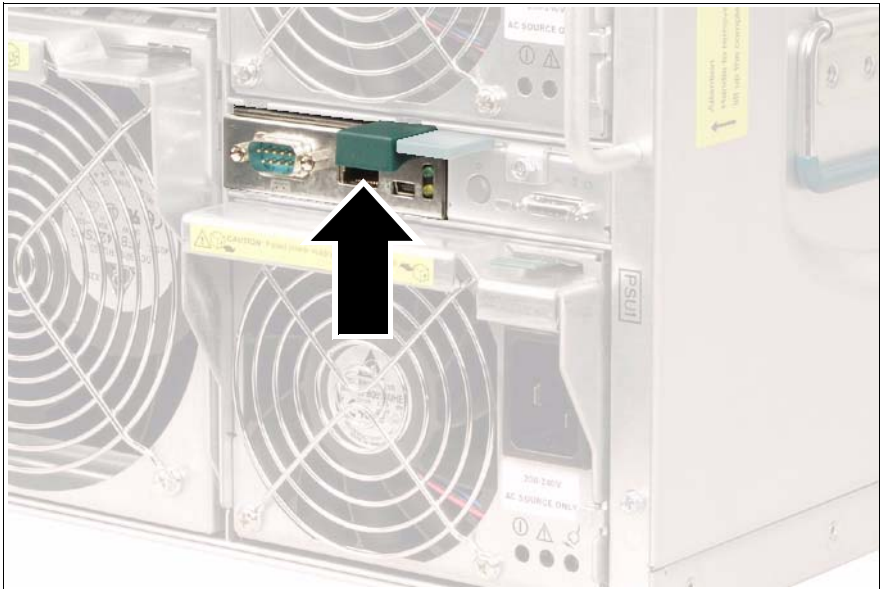
Figure 62: Disengaging the management blade
