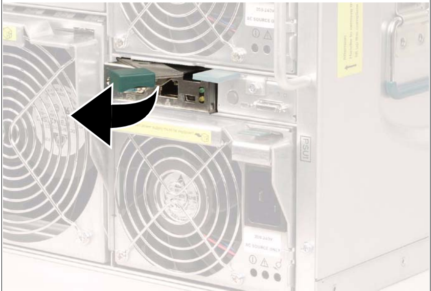
Figure 63: Disengaging the management blade
