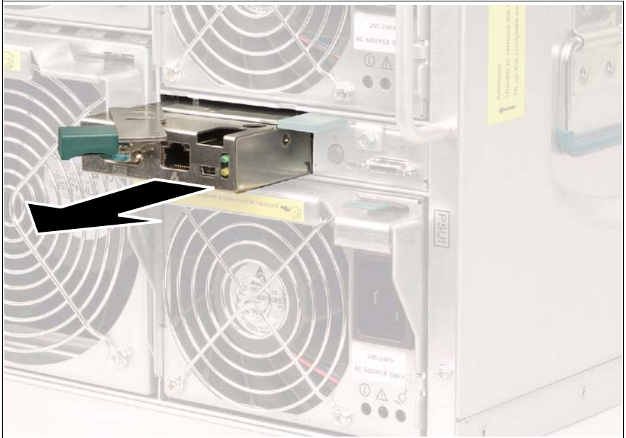
Figure 64: Removing the management blade
