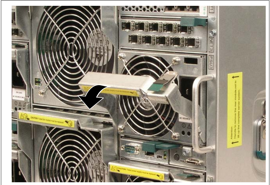
Figure 78: Removing the power supply unit
