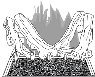
Figure 40 - Typical Flame Pattern
