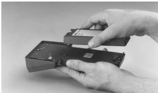
FIGURE 1-44. Memory Module Replacement.
