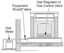
Figure 18 - Checking Gas Joints (Natural Gas Only)
