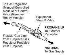
Figure 15 - Attaching Flexible Gas Line to Equipment Shutoff Valve
