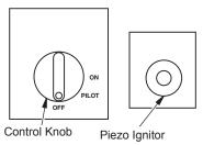
Figure 27 - Control Knob In The OFF Position
