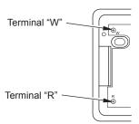
Figure 25 - Thermostat Base Terminals "W" and "R"
