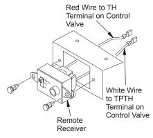
Figure 21 - Installing Remote Receiver
