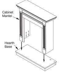
Figure 11 - Installing Cabinet Mantel onto Hearth Base
