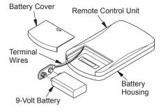
Figure 22 - Installing Battery in Hand-Held Remote Control Unit
