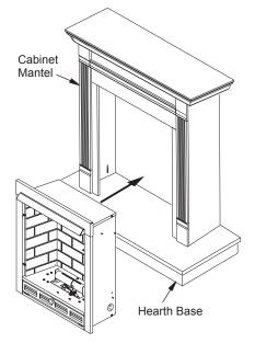
Figure 12 - Installing Fireplace into Mantel Assembly
