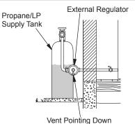
Figure 13 - External Regulator With Vent Pointing Down
