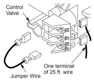
Figure 23 - Connecting Wire Terminals
