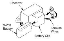
Figure 20 - Attaching Battery to Receiver
