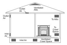
Figure 5 - Ventilation Air from Outdoors
