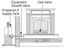
Figure 17 - Checking Gas Joints (Propane/LP Only)
