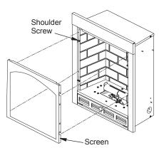
Figure 2 - Removing and Replacing Screen
