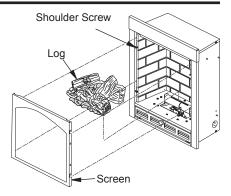
Figure 26 - Installing Log and Screen
