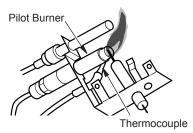
Figure 37 - Incorrect Pilot Flame Pattern (Propane/LP Remote-Ready Shown)
