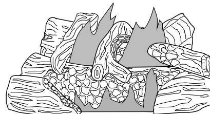
Figure 51 - Typical Flame Pattern for (V)T32 and (V)T36 Series Models
