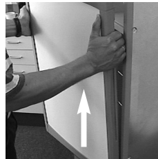
2. Take off the door by moving it upwards.
