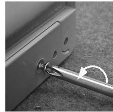
3. Unscrew the door strip (3 screws).
