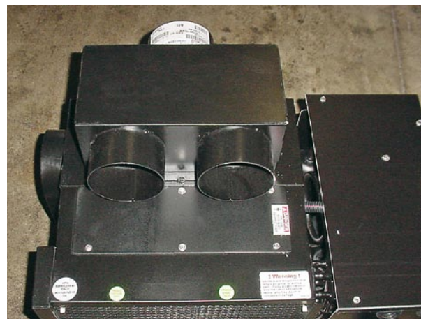
Figure 18b - Installing the air distribution plenum
