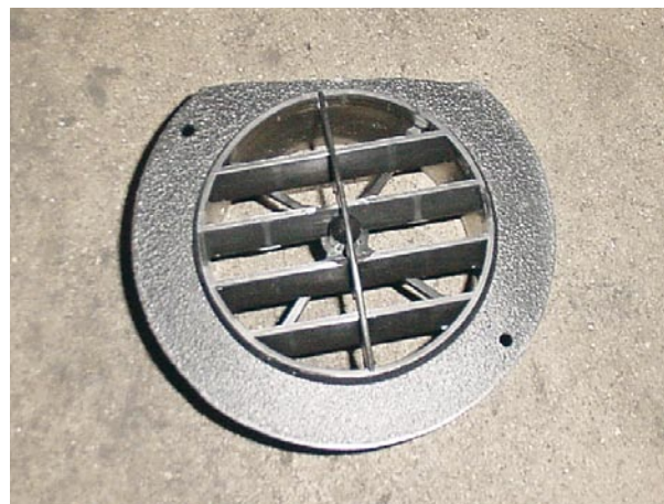
Figure 13 - First trimming cut on 4" grill
