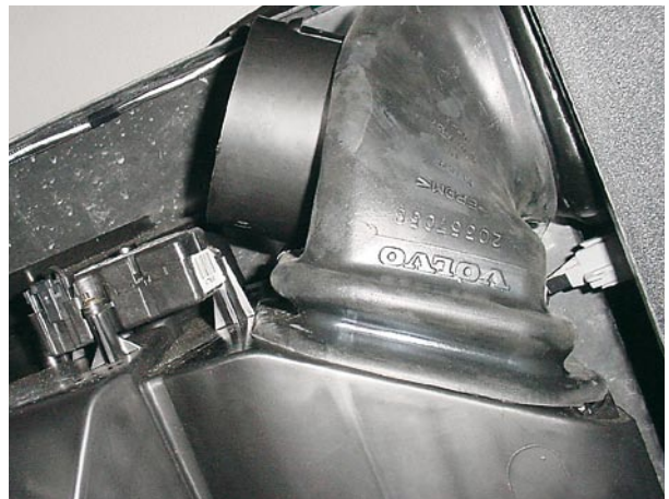
Figure 16 - Duct transition reinstalled
