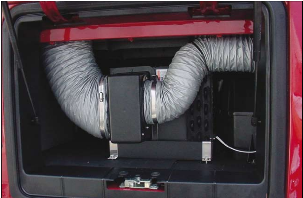
Figure 15. View of supply ducting connected.
