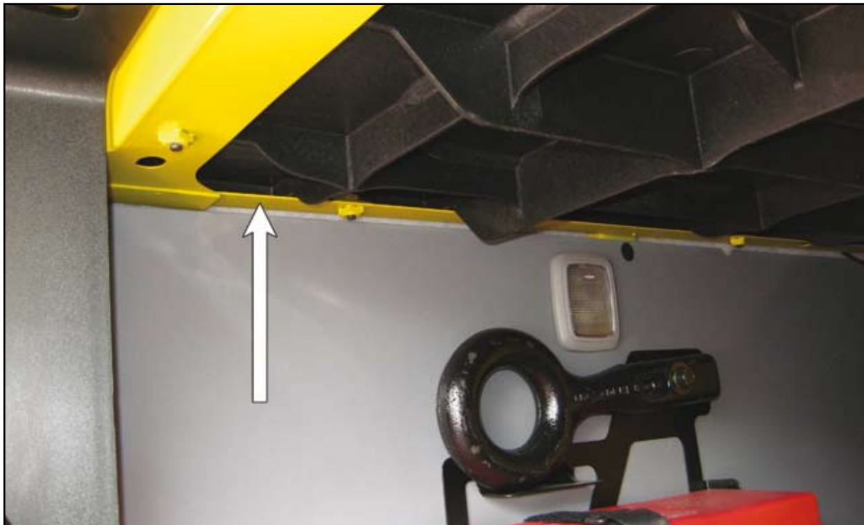
Figure 11. Location of cut out for ductwork.
