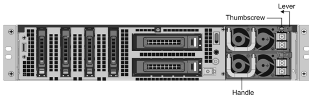
Figure 1-13. Removing the Existing DC Power Supply
