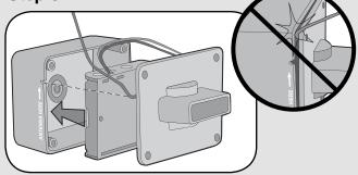
Insert battery pack facing away from circuit board and
