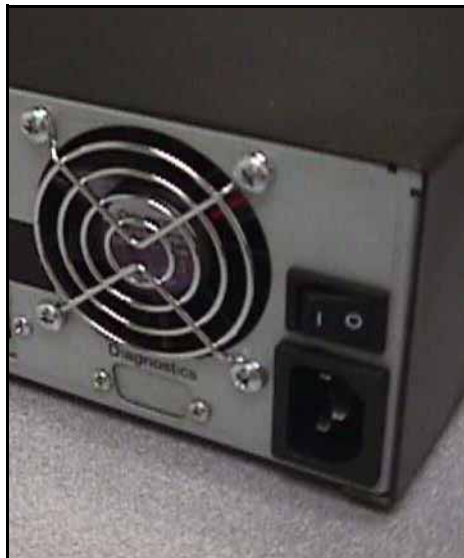
Figure 3-1 The DAStape power switch.
