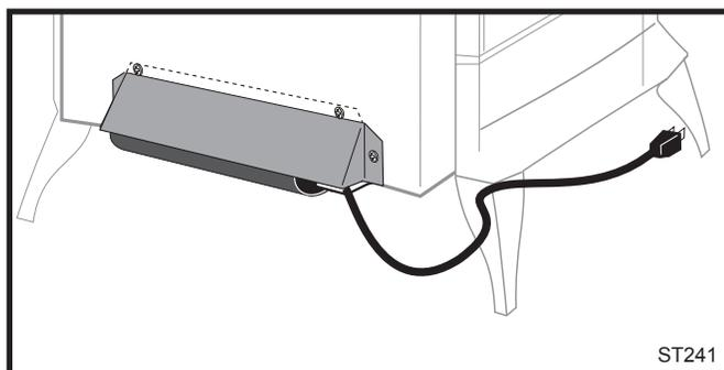
**Fig. 15** Correct position of fan skirt installation.
