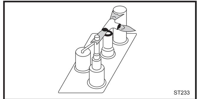
Fig. 48 Correct pilot flame appearance. PSE pilot.
