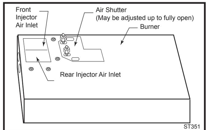
Fig. 40 Air shutter adjusted.
