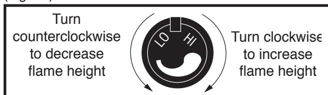
Fig. 47 Flame adjustment knob for Honeywell valve.
