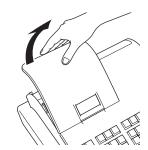
**2** Remove the battery compartment cover.
