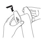
**6** Place the take-up reel into place behind the printer, above the roll paper.
