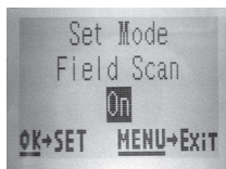
[Step 1] -set Field Scan Mode to “On”
