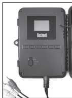
Cable from "A/V Out"
