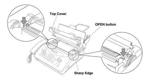
**3** Pull the jammed paper toward the back from the paper tray and remove it as per diagram A. If you can't, pull the jammed paper toward the front and remove it as per diagram B. If you cannot see any jammed paper, remove the ribbon cassette and check underneath. Remove any jammed paper.
