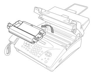
4 To clean the machine's thermal print head, wipe the metal and plastic part with a lint-free cloth that is dry or lightly moistened with isopropyl alcohol.
