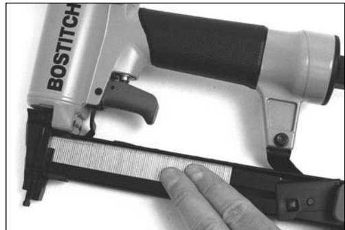
3. Pull back on red pusher handle; allowing pusher assembly to rotate clockwise. Slowly release pusher until it contacts the rear of the staple stick.
