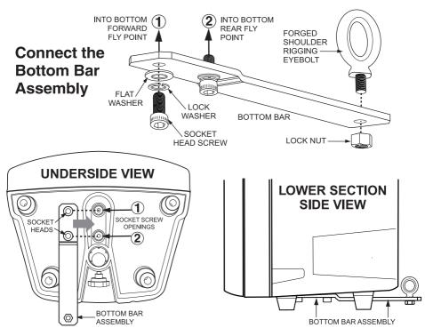
Attach the Bottom Bar Assembly to the underside of an AMT-Series Speaker as shown here.
