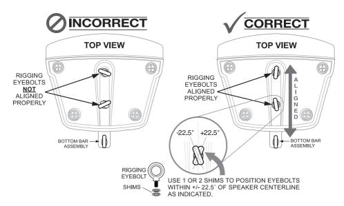
NOTE: Be sure that all hardware has been tightened securely. DO NOT over-tighten.
