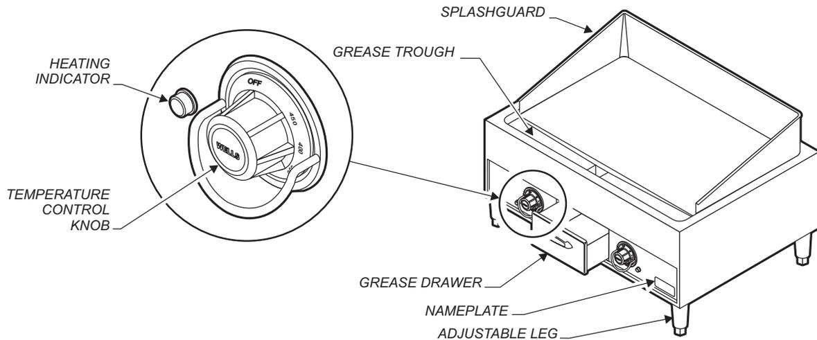
Fig. 1 Countertop Griddle Features & Operating Controls
