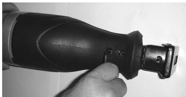
Using the Allen Key (67) to loosen the Set Screws (38) to adjust the Base Plate (44).
