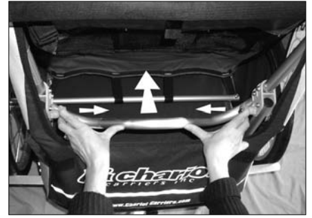
To fold the base, release both disks simultaneously and push the W-frame forwards.
