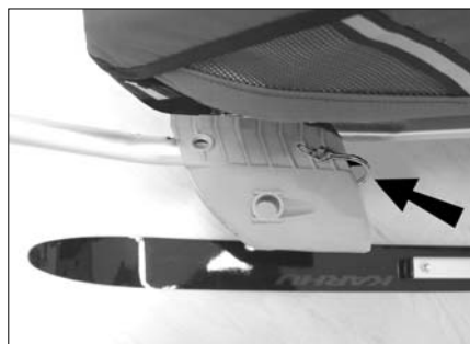
Once the holes of the attachment bracket and the drawbar are aligned with each other push the securing pin from below through bracket and drawbar and lock it by pushing the clip over the pin.
