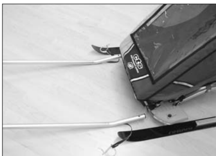
Slide the drawbar into the drawbar attachment bracket.
