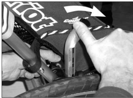
Pull the auto-lock disk and press the short, curved frame tube forwards.
