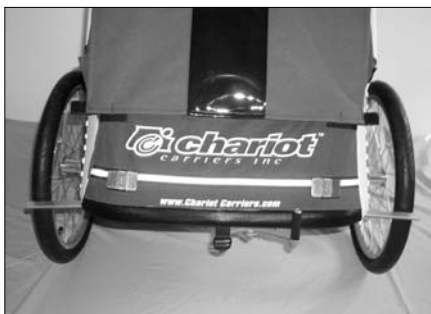
Plastic wheel on the Cabriolet, Comfort and Cheetah. Screw two reflectors onto each wheel at the corresponding brackets.
