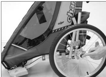
Fitting the skiing kit: Firstly, remove the wheel by pressing on the axle knob.
