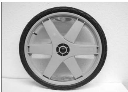
Plastic wheel on the Cabriolet, Comfort and Cheetah. Screw two reflectors onto each wheel at the corresponding brackets.
