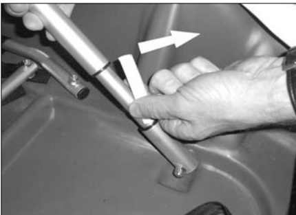
To continue assembly, first take off the transport safety lock.
