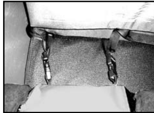
First connect the fastex buckles on the underside of the baby seat with their counterparts on the lap belt ends.
