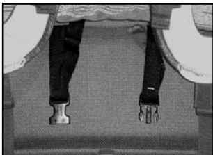
Arrangement of fastex buckles needed for centre-fitting of the baby seat Front view.
