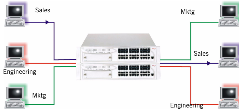
Figure 11.2 VLAN Switching and Bridging
