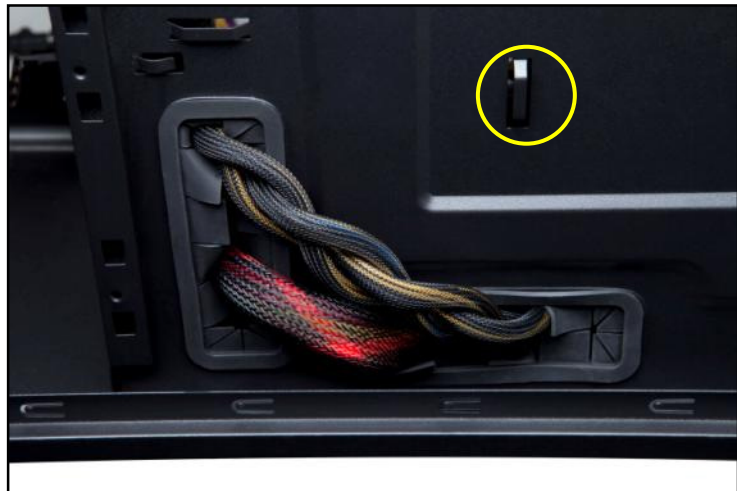
Using the grommet-lined cable routing holes to route PSU cables. The yellow circle shows a cable tiedown
