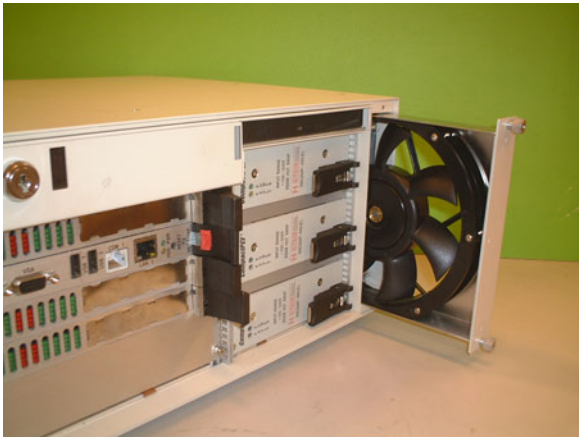
Figure 2.8: Hot-swappable fan maintenance
