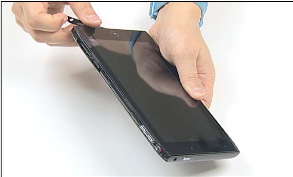
Figure 3-9. Releasing Right Cover (1 of 2)
