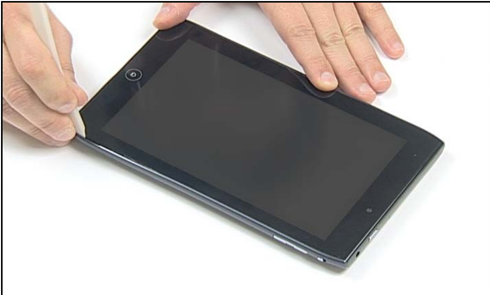
Figure 3-7. Releasing Top Cover (1 of 2)
