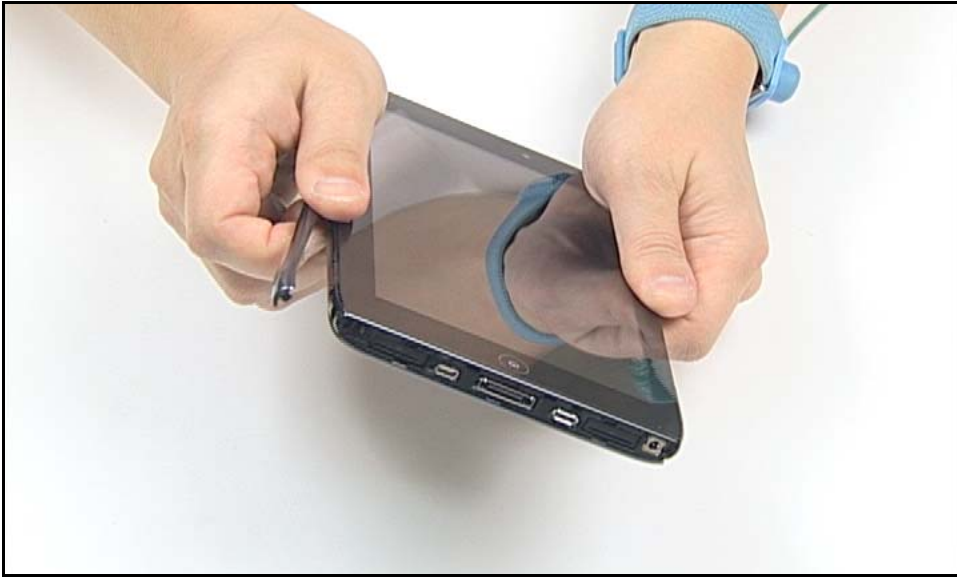
Figure 3-11. Releasing Bottom Cover (1 of 2)
