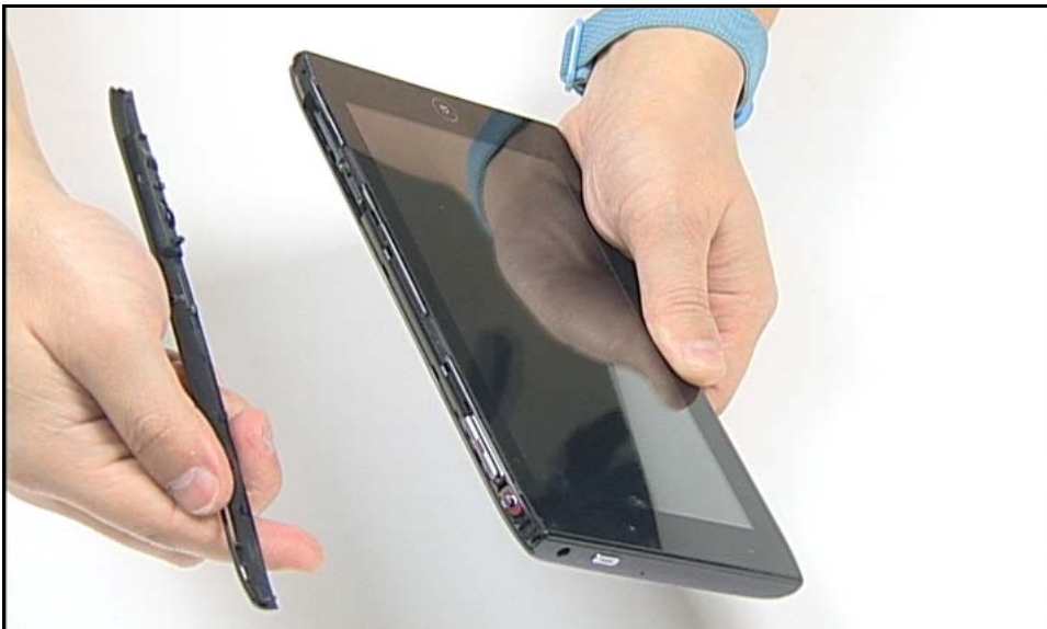
Figure 3-8. Releasing Top Cover (2 of 2)
