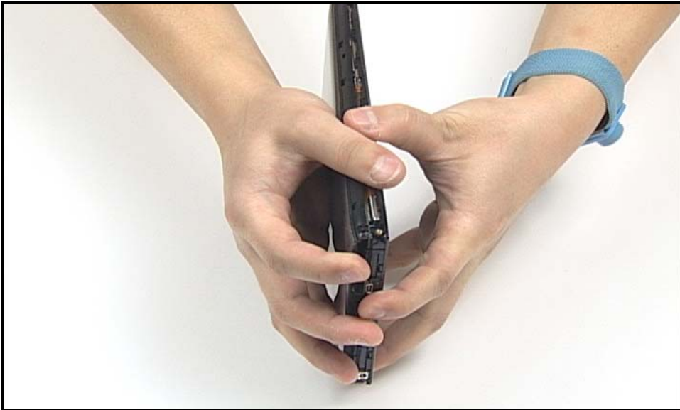
Figure 3-17. Removing Lower Case (1 of 3)
