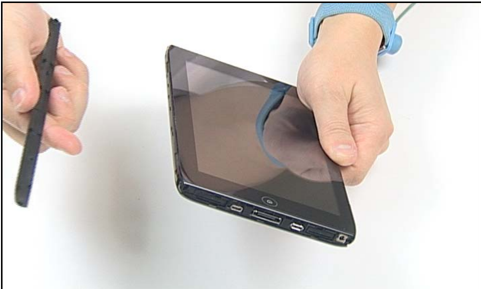
Figure 3-12. Releasing Bottom Cover (2 of 2)
