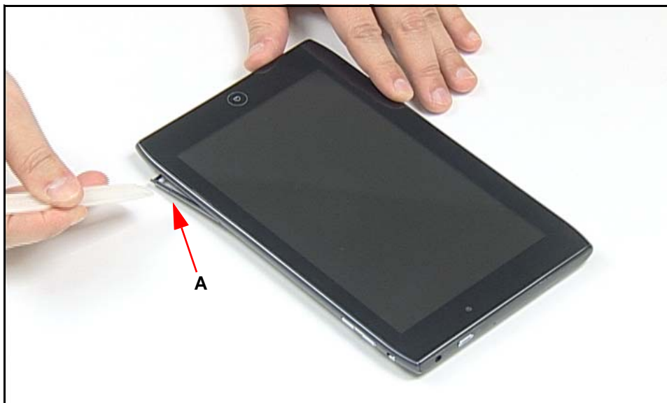
Figure 3-4. SIM/micro-SD Card Removal
