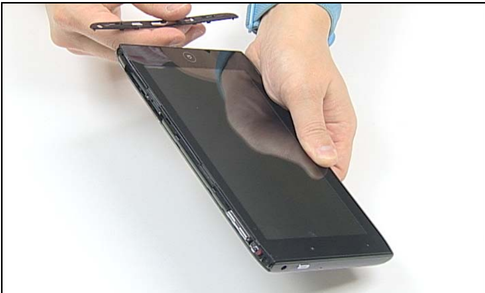
Figure 3-10. Releasing Right Cover (2 of 2)
