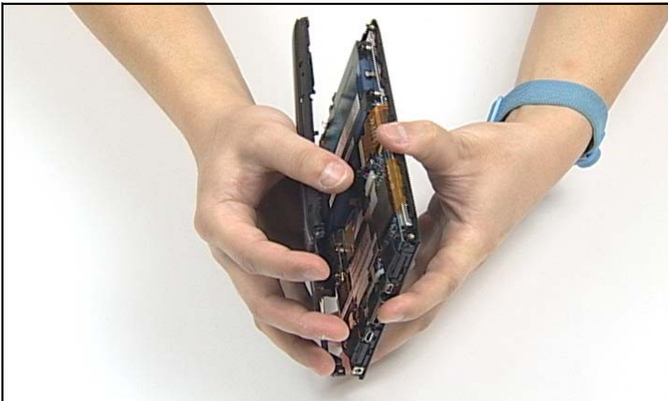
Figure 3-18. Removing Lower Case (2 of 3)
