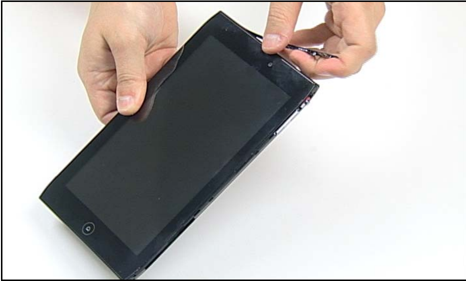
Figure 3-13. Releasing Left Cover (1 of 2)
