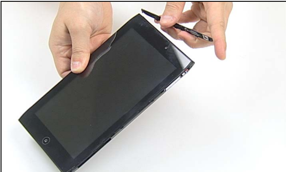
Figure 3-14. Releasing Left Cover (2 of 2)
