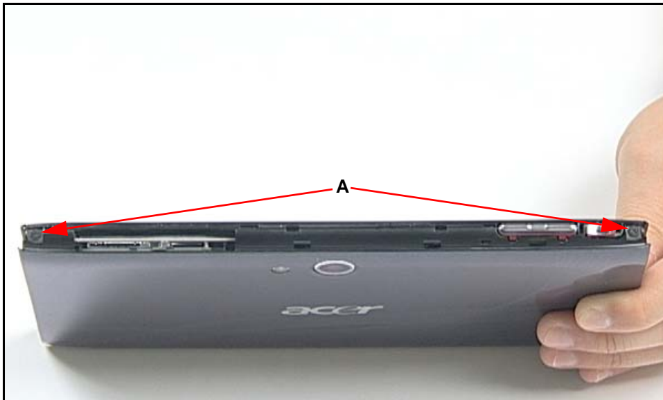
Figure 3-15. Bezel Screws (1 of 2)
