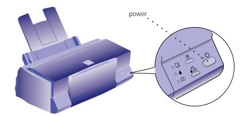
2. Plug the power cord into a properly grounded outlet. To protect the printer from power surges, you may want to use a surge protector.
