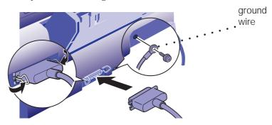
3. Connect the other end of the cable to your computer's parallel port and secure it as necessary.
