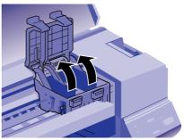
Open the ink cartridge packages. Completely remove the disposable yellow portion of the tape seal on top. Don't remove the white portion.
