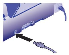
3. Connect the other end of the cable to either the printer port  $\stackrel{\frown}{\sqsubseteq}$  or the modem port  $\stackrel{\checkmark}{\leqslant}$  on your Macintosh.
