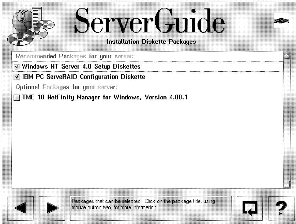
Figure 53. ServerGuide 3.0 Installation Diskette Packages. The Setup Diskettes package contains the three boot diskettes for NT 4.0. The TME 10 NetFinity package contains diskettes for TME 10 NetFinity Manager.
