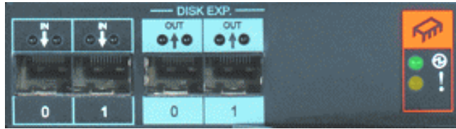
Figure 2-13 DS6000 expansion enclosure SBOD controller card
