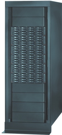
Figure 1-3 DS6800 with five DS6000 expansion enclosures in a rack
