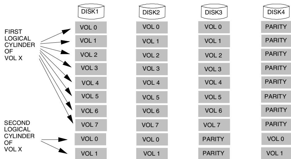
Figure 22. RAMAC3 Drawer Logical Volume Mapping
