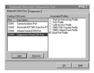
rectly installed the *Bluetooth* PCMCIA card and software). Click on any one of these ports and verify that the Serial Port Profile is checked. If it is not checked, then click the box next to **Serial Port Profile**.
