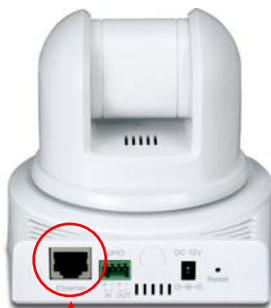
Connecting the Ethernet Cable
