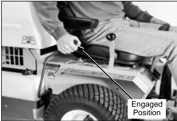
PTO Clutch Engaged (Model MD Shown)
