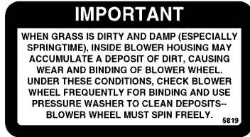
Top of Blower Housing (5819)
