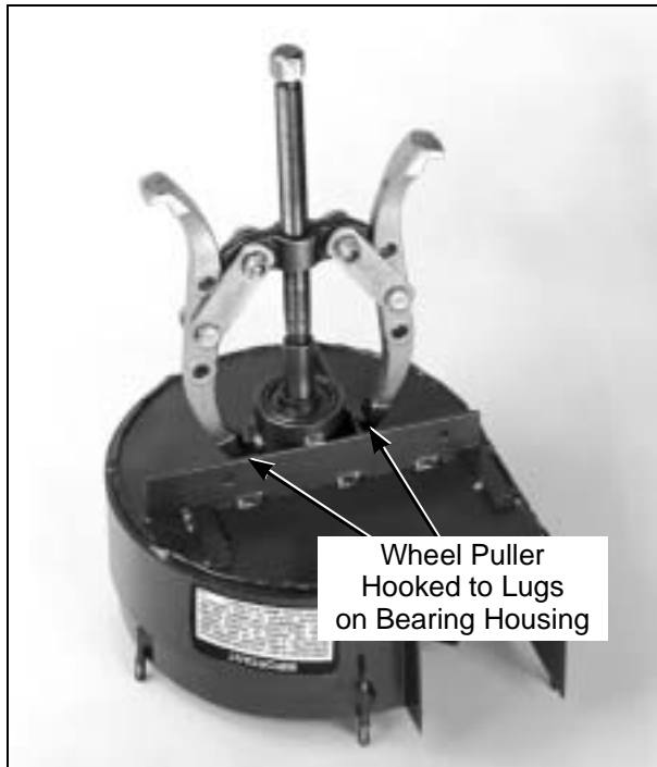
Pressing Blower Wheel Out of Housing
