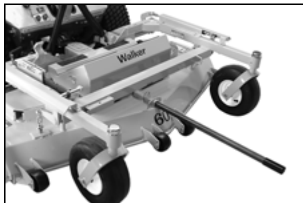
Tilt Bar Installed
