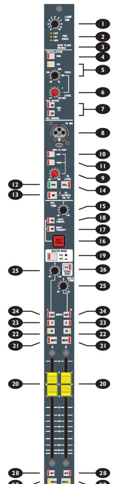
The function of the Output SOLO switch is also affected by the GLOBAL MODE (STE) switch. If the mode is mono, each Output SOLO button switches an equal feed at unity gain to each of the AFL left and right busses, and a PFL signal to the PFL bus. If the mode is stereo, the SOLO switches are logic linked as a pair and the AFL feed is changed to stereo, at unity gain. The PFL feed remains mono.
