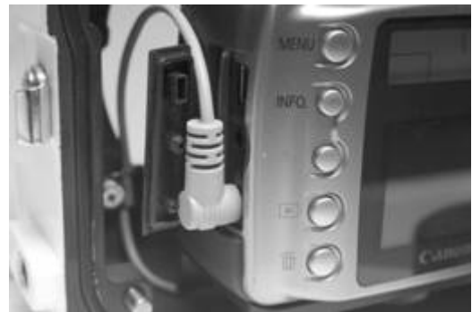
Picture B: Trigger release cable position
