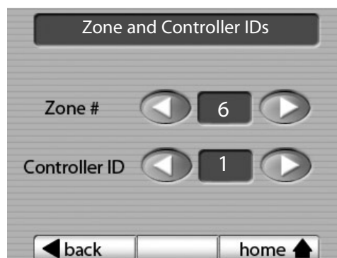
This screen is shown when "Zone and Controller ID" is selected
